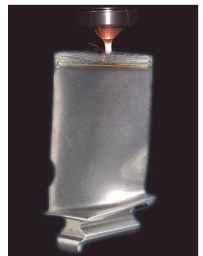
Blade with Laser Metal Deposition
