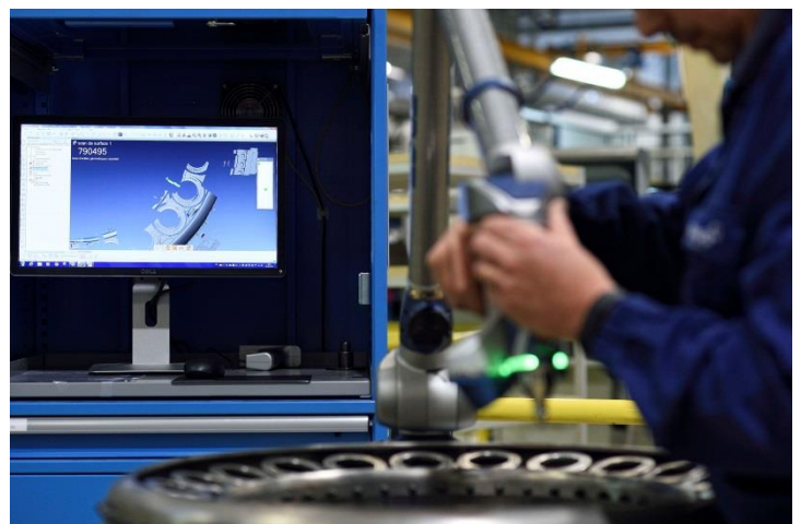
Parts measurement by 3-D scan
